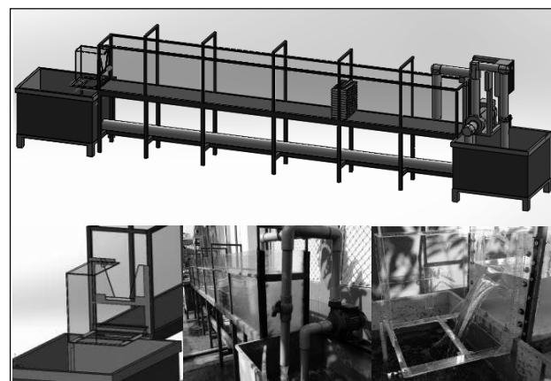
Fig. 2. Open water tunnel at width 0.39 m, high 0.40 m, and long 4.80 m
