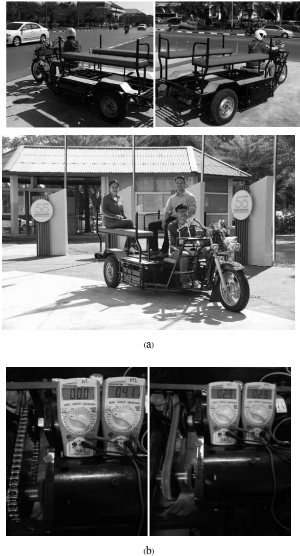
Fig. 8. Test of the proposed simple dual DC motor drive system: (a) driving tests and (b) speed-resistive control for one-two operating motor(s) control
