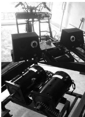
Fig. 3. Photographs of the dc motors ZC4-48 used for the prototype vehicle
