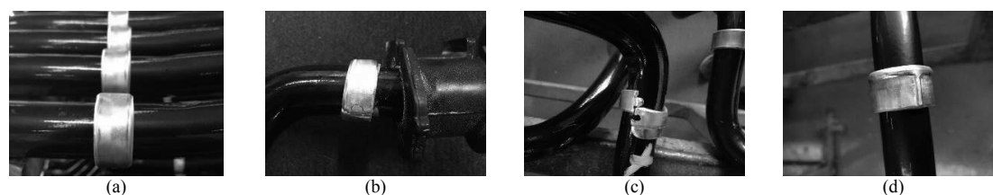
Fig. 3. Characteristics of standardized products (a) and non-standardized products, (b) stopper ring's skewness, (c) misalignment of the stopper ring's cogs, and (d) deformed stopper ring from the pressure.
