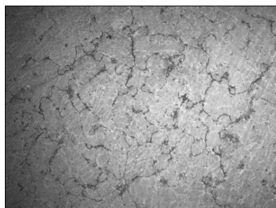
Fig.1 The optical micrograph(100x) of as-cast showing significant heterogeneously dispersed manganese carbide at grain boundary
