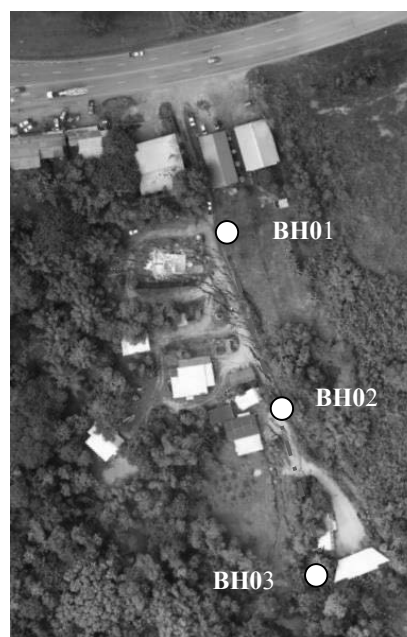
Fig. 3 Digital Ortho-rectified image and borehole positions
