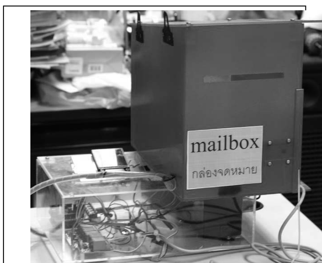
Fig 6 Picture of postal alert and security system via line application.
